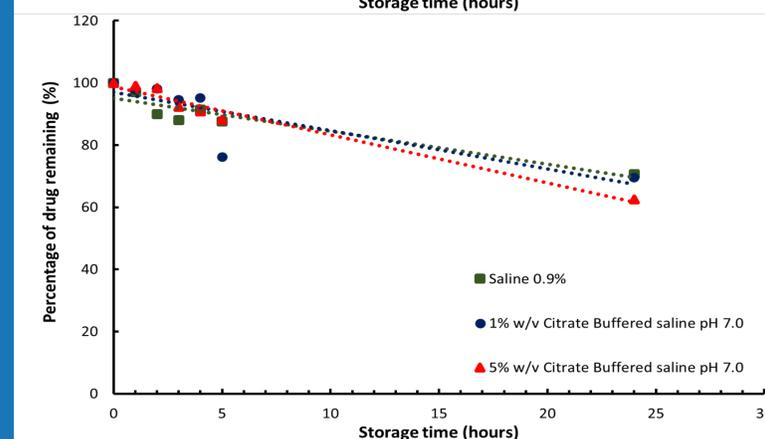
**FIGURE 2.** Degradation rates of high concentration (c. 25 mg/ml) meropenem at 32°C in different buffered diluents.
