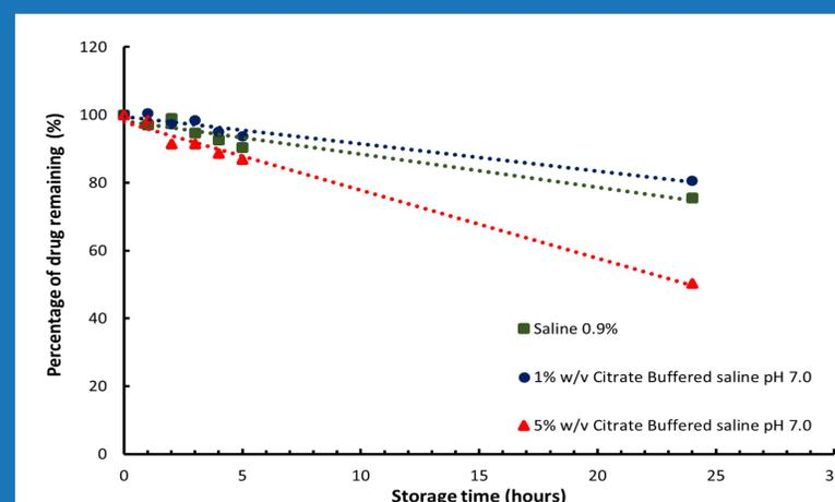
**FIGURE 1.** Degradation rates of low concentration (c. 6.25 mg/ml) meropenem at 32°C in different buffered diluents.
